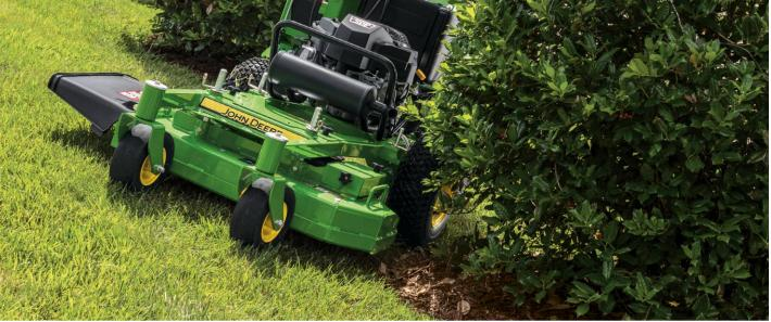
**Better weight distribution means better operation.** We significantly improved the weight distribution on the M & R series to help operators on mowing slopes or tricky side-hills. Combine with our easy-to-use controls, operators can hold the line on hillsides.
