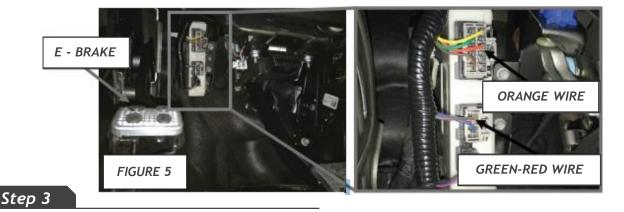
Attach 6" wire between ORANGE wire (pin 3 on C2498C connector and GREEN-RED wire (on F150) or RED wire (on Super Duty) (Pin 1 on C2498A connector) using Scotch-locks (for F150 supplied scotch-locks can be used, Super Duty are not supplied, recommend using 3M 902). This will activate a continuous +12V to the +12V power pin on the 7 pin trailer connector. Refer to figure 6.
