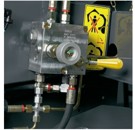
Variable bale density in the ROLLANT 340. The right bale density for different crops is set independently by adjusting the hand wheel.
