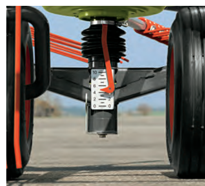
Keeping it flexible, with the rake height adjustment scale.
