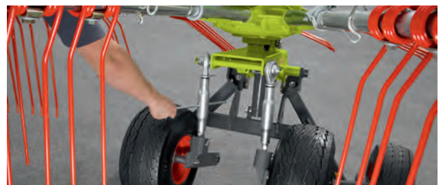
The unique chassis design of the CLAAS side delivery rake allows lift heights of up to 28 in (70 cm).
