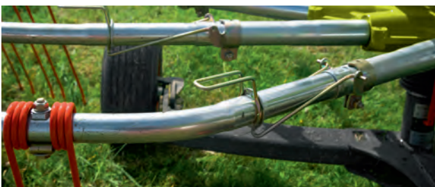
In the event of a collision, the tine arms snap off at a set bending point, preventing any serious damage.
