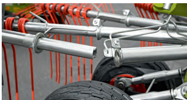
Lemon profile attachment and PROFIX tine arm attachment system in the LINER 700 TWIN.
