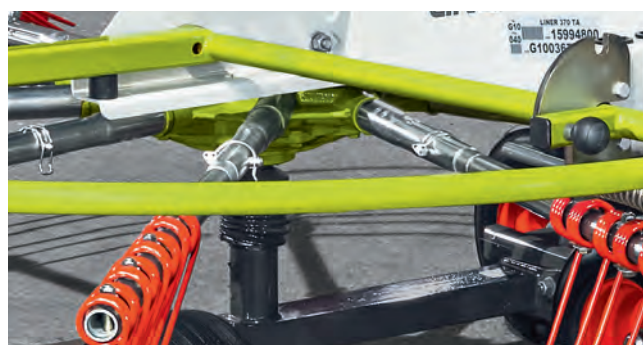
Lemon profile attachment and clamping splint in the LINER 370 T.
