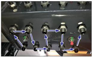
Clamp from the outside to the inside (the figure shows the left rear axle, lower side)
