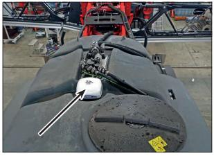
GPS receiver mounted on spraying mixture container
