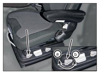
Under certain operating conditions it is advantageous to switch on the horizontal suspension. This enables the driver's seat to better absorb impact loads in the direction of travel.
