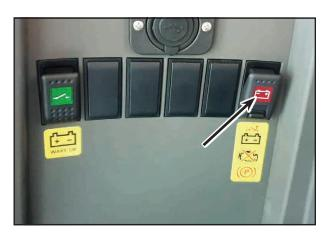
The red switch is used to shut off the current supply early. The battery is disconnected from the vehicle electrical system without overrun time. The diesel engine shuts itself off. The exhaust gas treatment (optional) keeps running for another 15 minutes until final shut-down.
