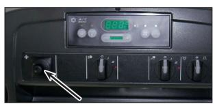
Switch for adjusting the outside mirrors
