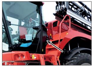
Mechanical release device of access ladder
