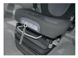
The seat depth can be individually adjusted. Pull the right handle up to adjust the seat depth. The desired position is reached by simultaneously pushing the seat area forward or backward.
