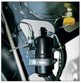
Dryer cartridge pressure switch
