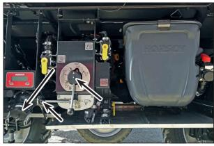
Filling port for spraying mixture container and pressure side valve
