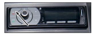
Briefly press the power button to turn on the unit. Press and hold the power button for one second to turn it off.
