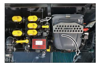
Flush the respective preparation through the illuviation valve into the water of the spraying mixture container. A difference is in this case made between the illuviation of fluid and powdery preparations or carbonyl diamide.
