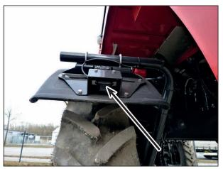
Wheel camera on the right front wheel fender
