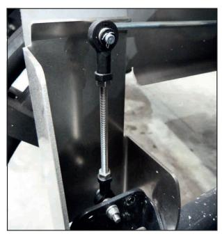
Folding boom level suspension hooked up
