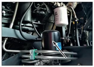
Compressed air system dryer cartridge
