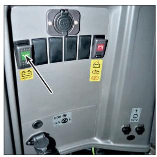
Main battery switch for power supply
