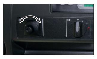
> Turn the switch up, down and to the side until the outside mirror is optimally adjusted:
