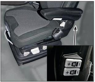
By pressing the Plus or Minus switch on the rear of the backrest, the bulge of the backrest can be adjusted individually.
