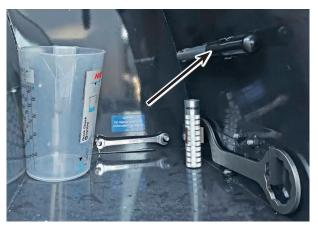
Mechanical release device actuating lever
