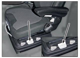
The respective driver's weight must be adjusted with the vehicle stopped and the driver's seat loaded by briefly pulling the automatic weight and height adjustment lever. Sit absolutely calmly when making the adjustment.
