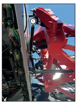
The slope compensation consists of two hydraulic cylinders that are locked or unlocked via lock valves.
