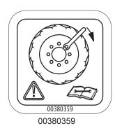
Tighten with torque of 510 Nm [375 ft lb]
