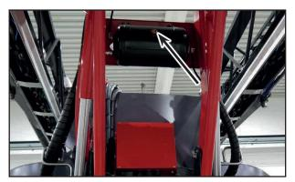
Parallelogram air reservoir with drainage valve
