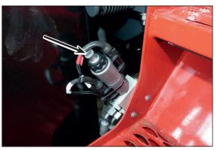
Valve for mechanical release of access ladder
