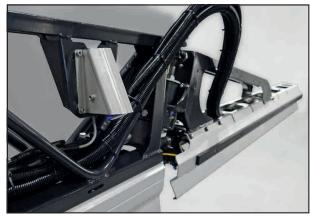
Ultrasonic sensor on the folding boom
