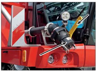
Direct filling port (right side of machine, filter optional)
