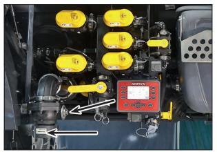
Filling port for spraying mixture container
