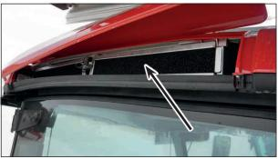
Activated-carbon filter with pocket filter
