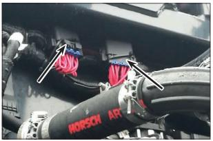
Position of pulse width modulation fuses
