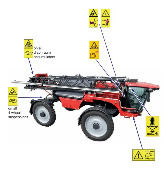
Safety stickers with the addition "2x" can be found on either side of the machine.
