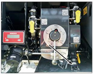
Port for water systems Basic and CCS fresh water tank
