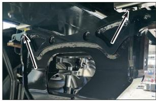
Lifting device with mounting bracket
