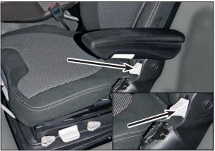
Pull the lever up to adjust the backrest. Do not press against the backrest while unlocking it. The desired position is reached by simultaneously loading and unloading the backrest. Release the lever to lock again.
