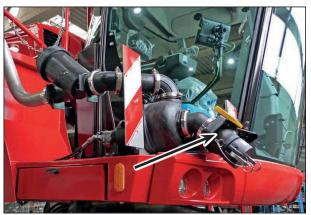
Direct filling connection with pump and filter (optional)
