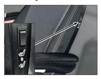
The seat heating is switched on by flipping the switch on the left side of the backrest upward. The seat heating is switched off again by returning the switch to the centre position 0.
