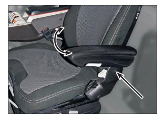
The left arm rest can be folded back and adjusted in height, if required.
