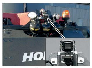
Rear view camera in folding boom middle section
