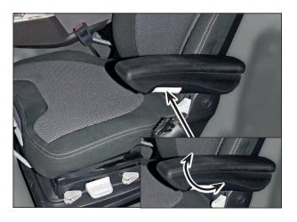
The longitudinal inclination of the arm rest can be changed by turning then hand-wheel. Turning towards the outside lifts the armrest at the front, turning towards the inside lowers it at the front.
