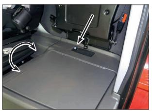
Storage compartment with integrated cooling function under the seat area of the instructor's seat.
