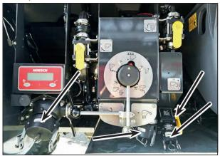
Filling ports of water system Basic and water system CCS
