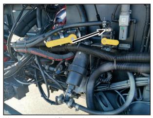
Water separator and filter-regulator combination
