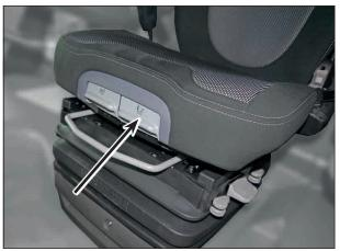
The inclination of the seat area can be individually adjusted.
