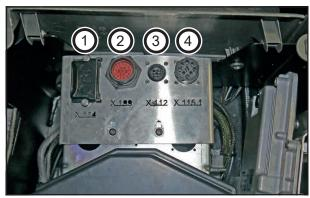
Vehicle socket outlets (the figure shows emission standard stage 5, machines with emission standard 3a have a different vehicle socket for engine diagnostics (4))
