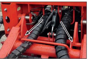
Parallelogram interlock locked (sample figure)
