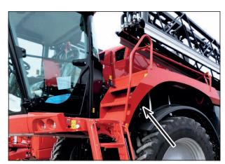
Compressed air system dryer cartridge position
