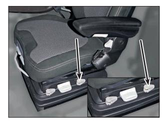
Under certain operating conditions it is advantageous to switch on the lateral horizontal suspension. This enables the driver's seat to better absorb impact loads from the side.
