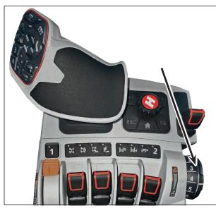
Manual correction for drift on a slope
