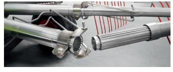
**PROFIX tine arm bracket.** The patented PROFIX tine arm bracket with multiple splines keeps the tine arms firmly attached. Additionally, in a collision, the predefined bending point protects the rotor assembly from damage.
