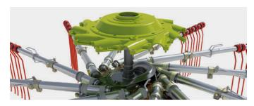
Continuously lubricated rotor housing assembly. The rake's rotor housing is filled with oil and hermetically sealed so that the transmission is protected from dirt and maintenance-free. The cam rollers operate smoothly in an oil bath for frictionless operation and maximum service life.
