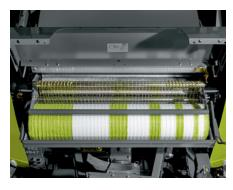
wrap provides coverage 2-3" over the edge of the bale for more secure binding and easier transport. Plus, with the optional COMFORT tying system, the operator sets the number of wraps from the cab to reduce waste on lighter crops.
