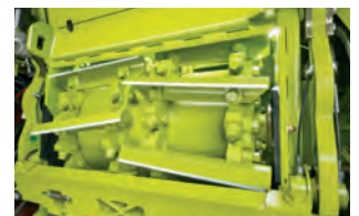
V-MAX chopping drum with knives removed.
