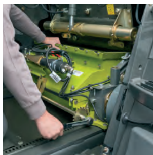
Quick removal and installation of the corncracker
