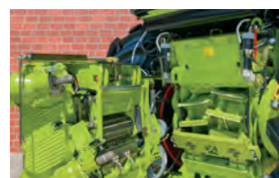
QUICK ACCESS: rapid access to the V-MAX chopping cylinder
