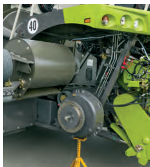
Quick removal of accelerator
