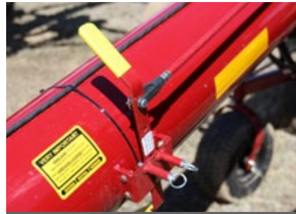
Reversible Gearbox Shifter
