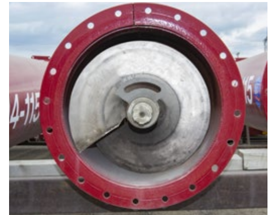
Fastened Spline and Hub Connection
