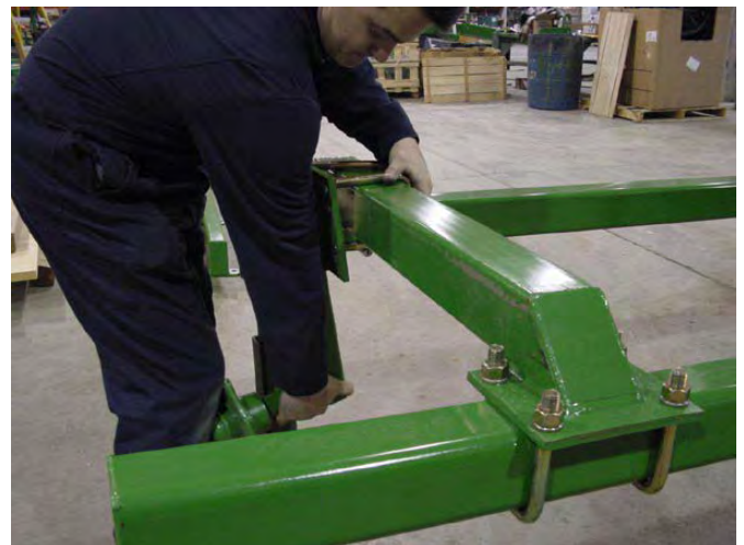
25. Install Wing Axle.
