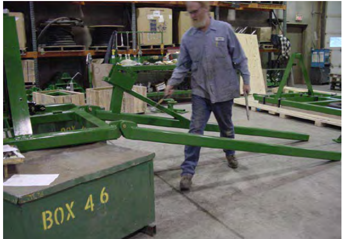
17. Left hand Wings attached.
