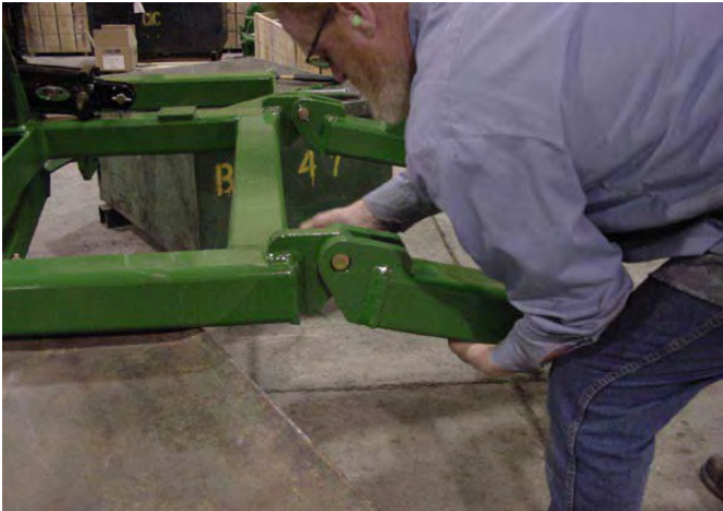
16. Connect from Wings to Center.
