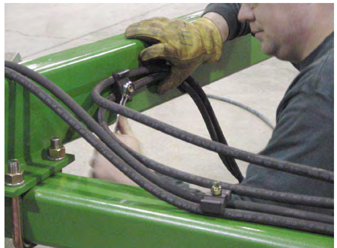
43. Route hoses forward, secure with clamps.
