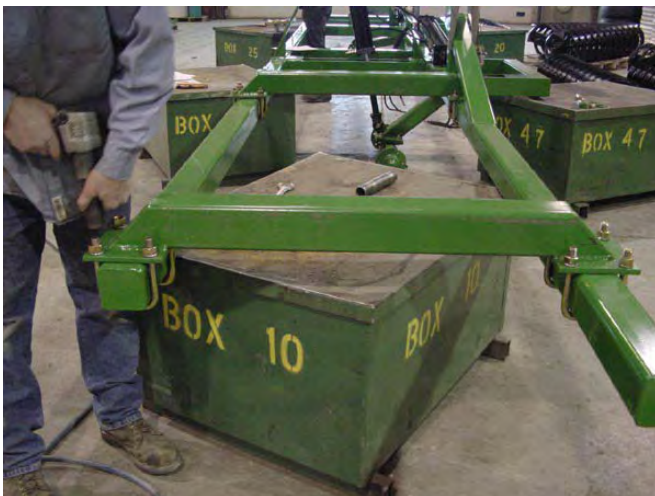
24. Align Wings with Center, tighten u-bolts.
