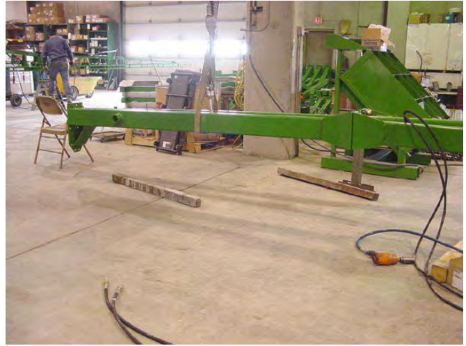
37. Install Hitch Extension.
