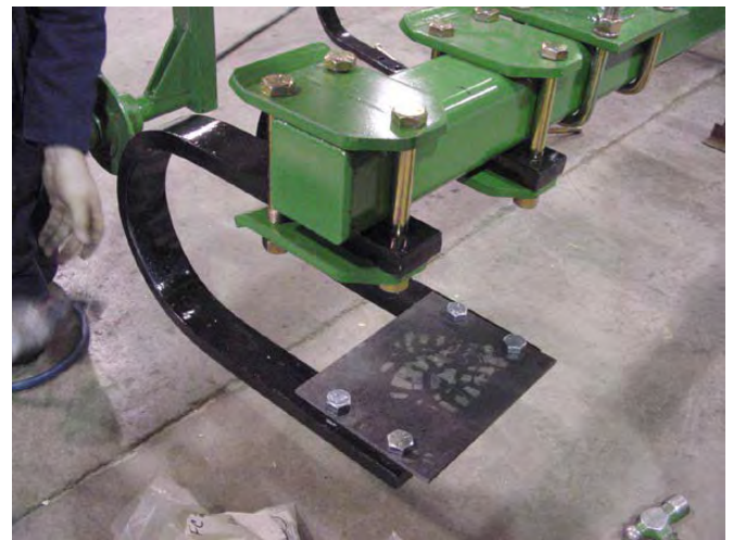
50. Tighten C-Shank mounting hardware.
