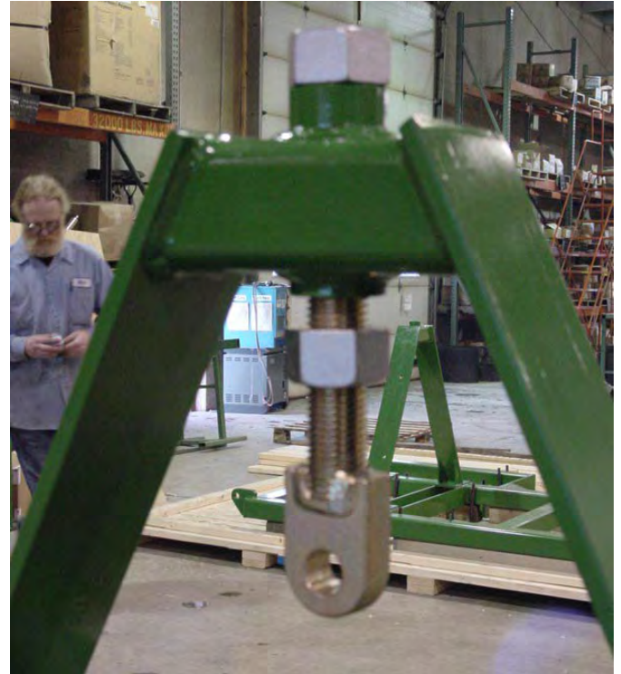
2. Install main and wing lift cylinder eye bolts (middle of adjustment).
