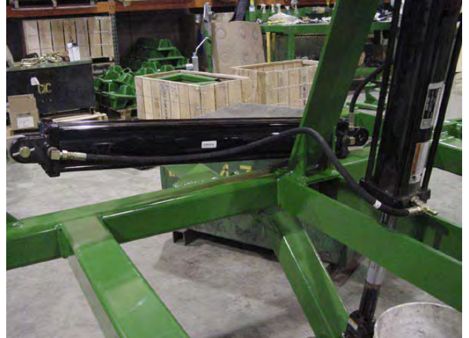
31. Hydraulic hose - Main and Wing Cylinders.
