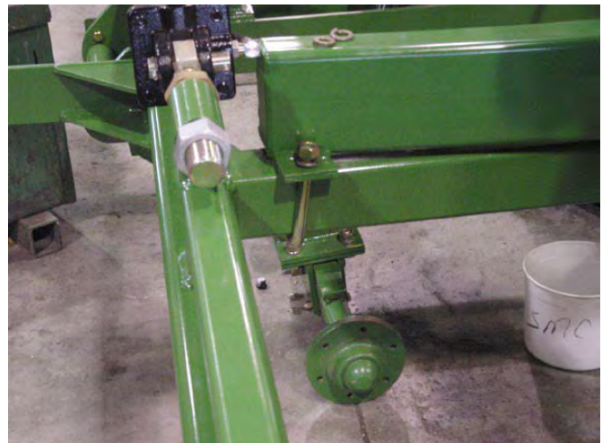
35. Rear u-bolt installed.
