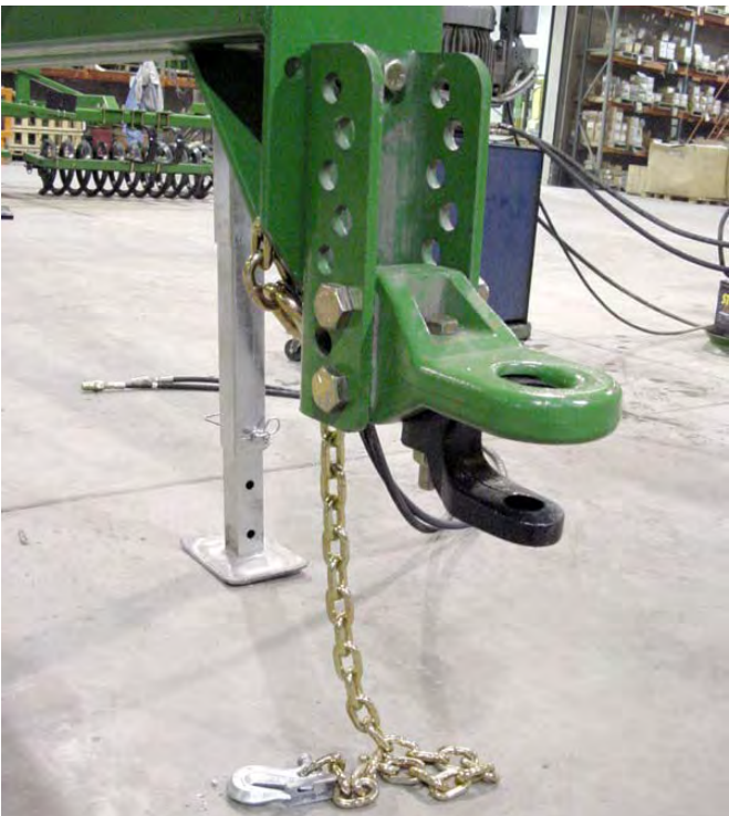
37. Install Hitch Extension.
