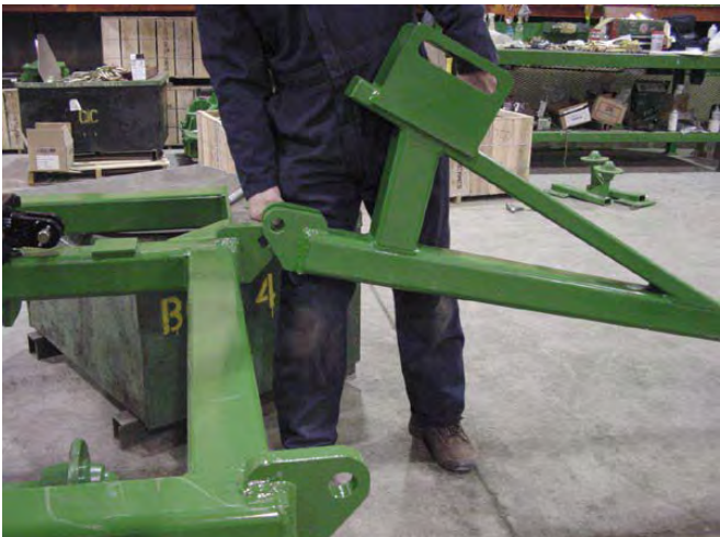
14. Connect rear Wings to Center.
