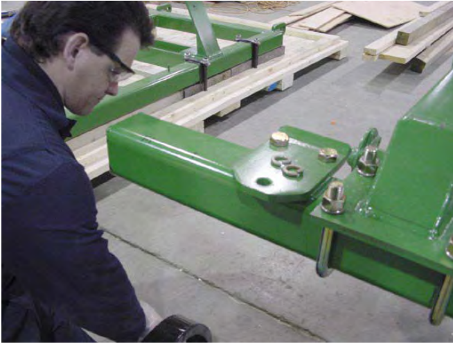
47. Mark frame using layout drawing, located clamps.
