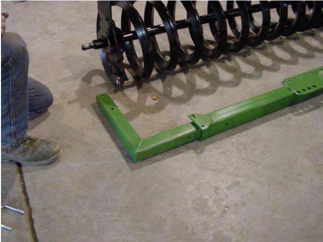
51. Lay out Coils and Pull Frames.
