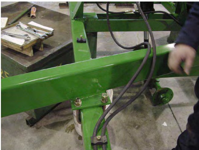
34. Attach Hitch Tubes to Center.
