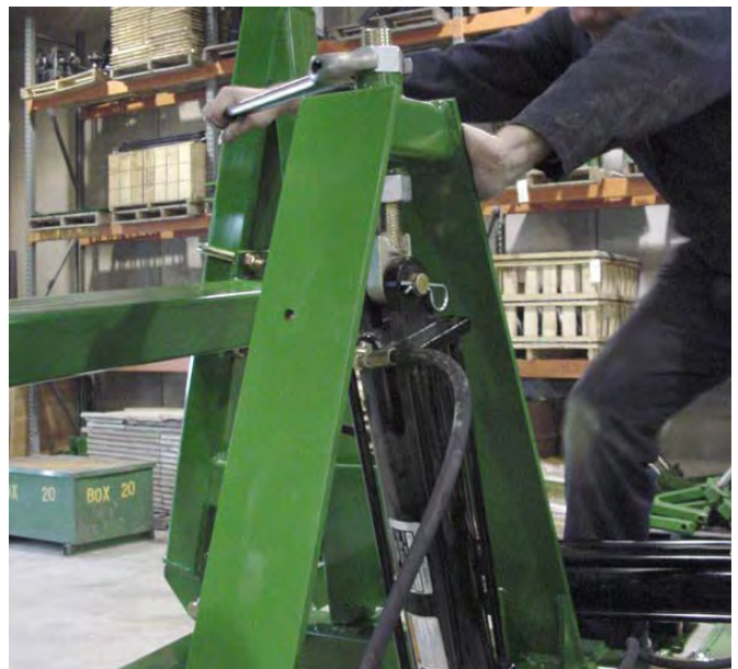
45. Adjust eye bolts so Wing rests on Center.
