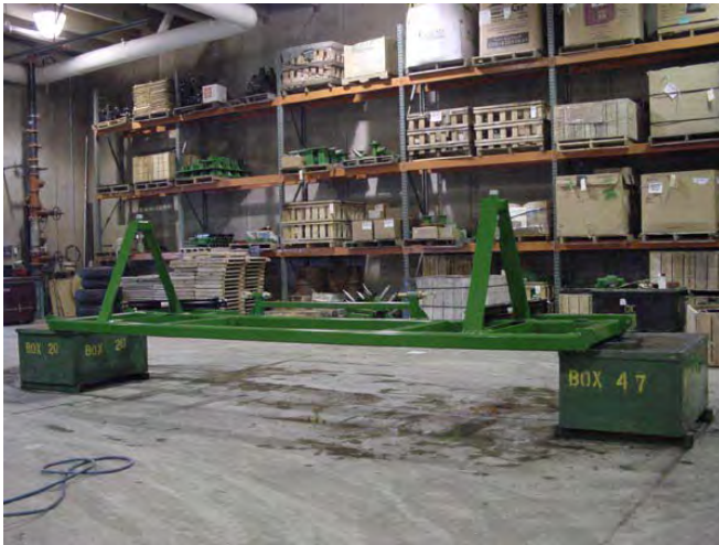
1. Position Center Frame on supports.
