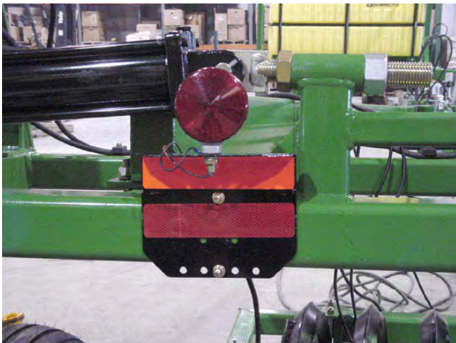
71. Rear Red Light installed.
