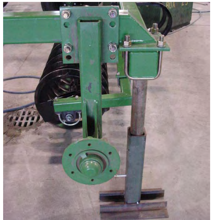
25. Install Wing Axle.
