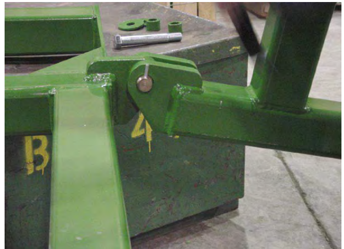
15. Install wing pivot pins, secure with roll pins.
