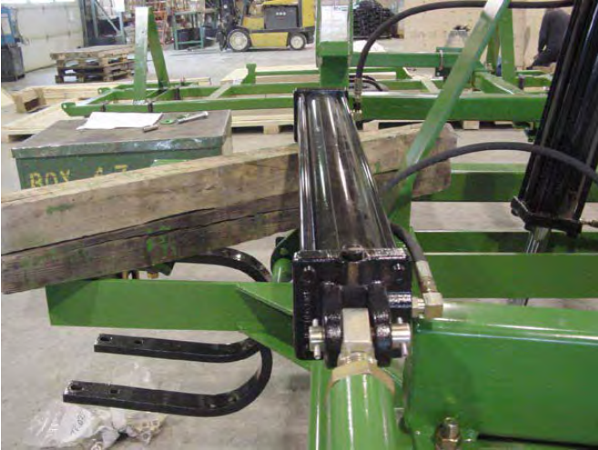
44a. Extend and retract wing lift cylinders.
