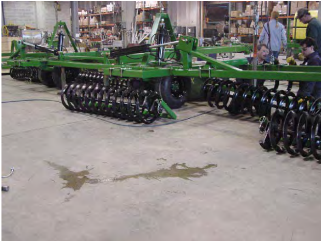
58. Roll Coil assemblies into position.
