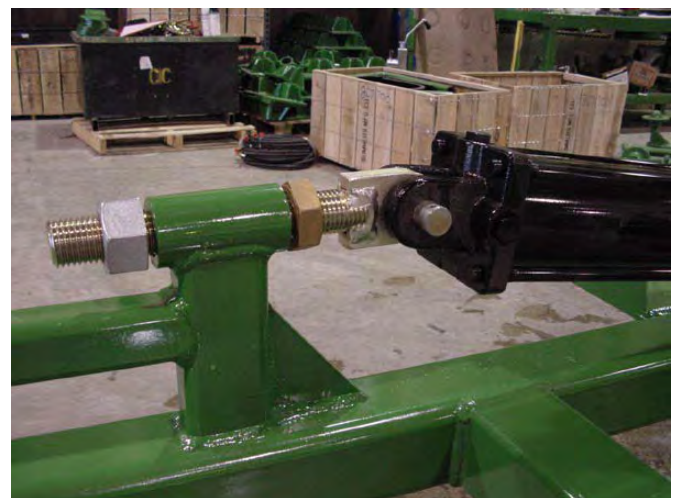
4. Attach wing lift cylinders.
