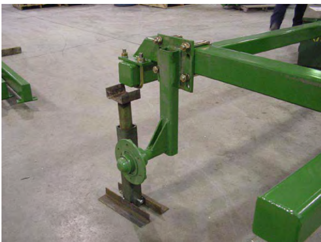
26. Left hand Wing Axle installed.
