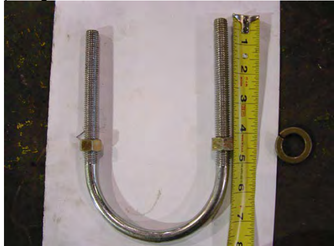
54. Pre-assembly of 1/2" nuts on bearing attach u-bolt.
