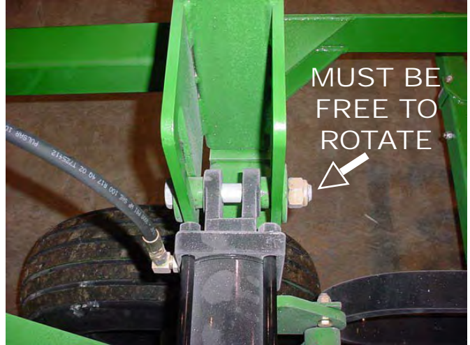
44b. Attach rod end of wing lift cylinders.
