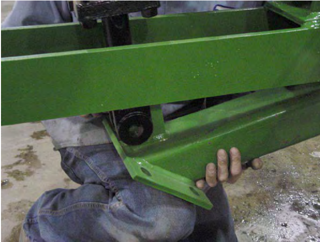
10. Connect rod end of main lift cylinder.
