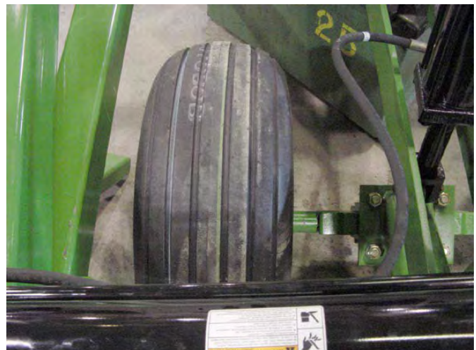
43. Route hoses forward, secure with clamps.
