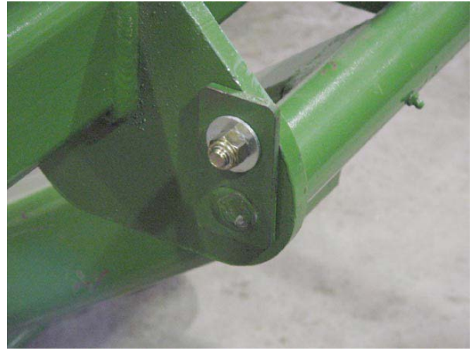
5. Install Center Lift Arms and secure Pivot Pin with bolt, washer and lock nut.
