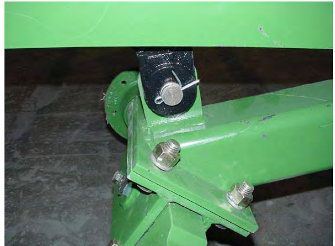
13. Walking Axle Assembly installed.
