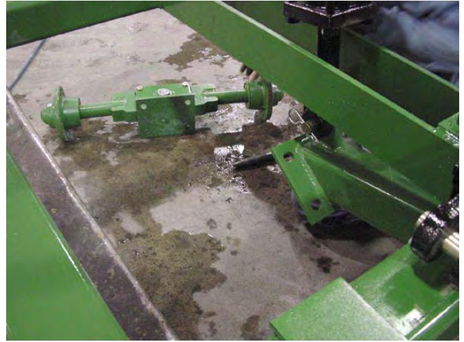
11. Position Walking Axle assembly.
