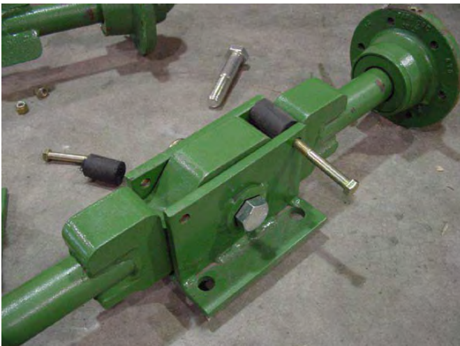
8. Install pivot dampeners.
