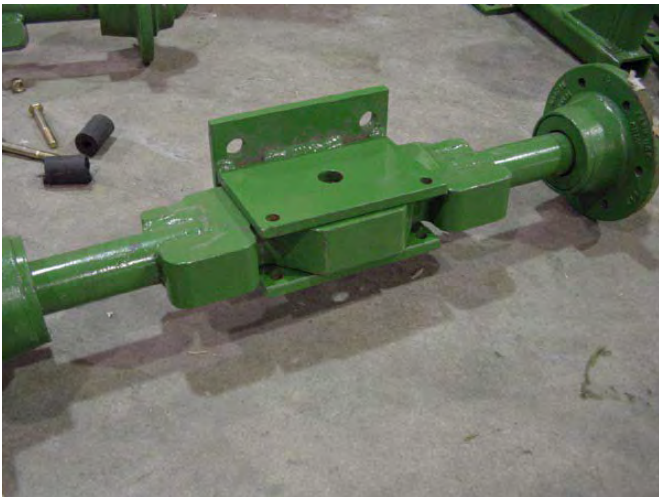
6. Assemble Walking Axles.
