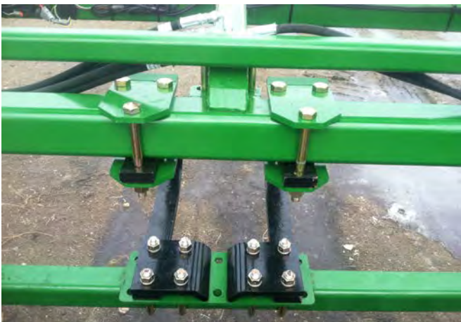
58. Roll Coil assemblies into position.
