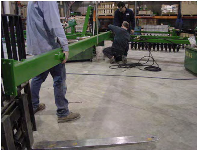
32. Install Hitch Tubes.
