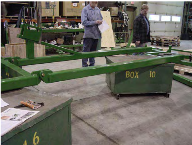
18. Left hand Wings leveled for further assembly.
