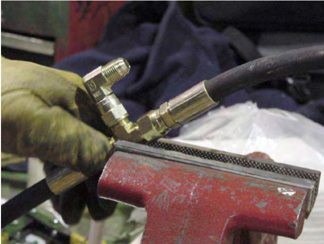
40. Pre-assemble front center fittings.
