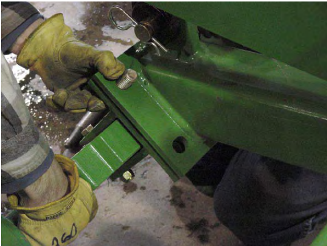
12. Secure Walking Axle to Lift Arm.
