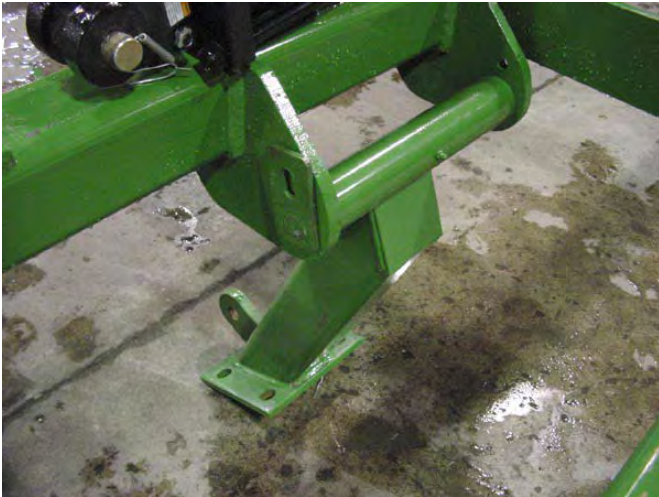
5. Install Center Lift Arms and secure Pivot Pin with bolt, washer and lock nut.
