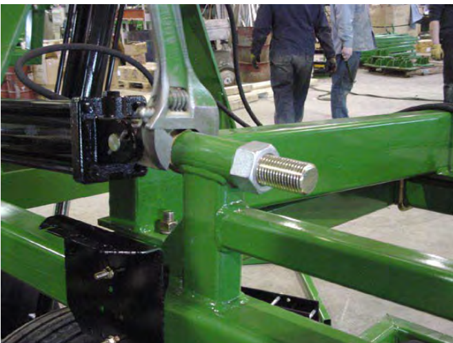
46. Tighten Wing Lift Cylinder eye bolts (above).
