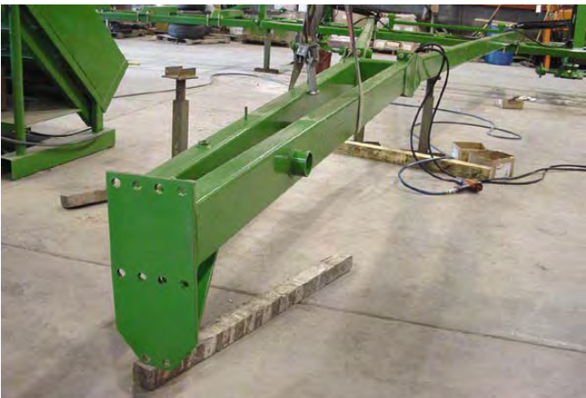
37. Install Hitch Extension.
