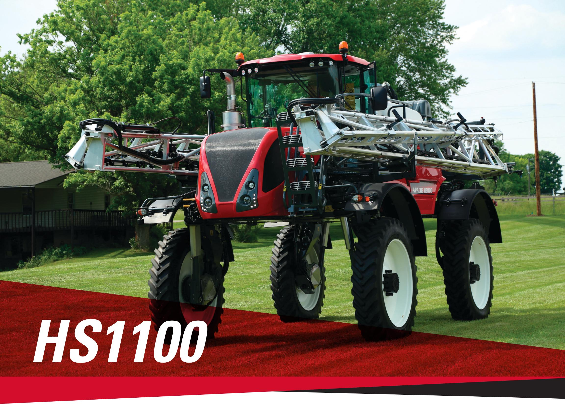
Engineered for those seeking performance, crop clearance, ease of use, and flexibility—all with an industry-leading 5-year warranty. Lighter than the competition, it adjusts automatically from 60 to 70 inches, making it the tallest rear boom sprayer in North America.
