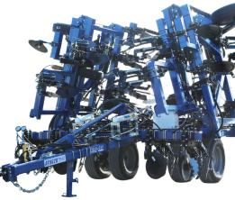
The Blu-Jet<sup>®</sup> AT6020 pull-type NH3 applicator is ideal for professional producers and commercial applicators that require high-acreage coverage and high-rate nutrient application. With a robust frame and toolbar design, working widths from 62.5' to 45' and innovative options that allow you to tailor the AT6020 to your needs, you'll be sure to get the job done during the narrow application window.
