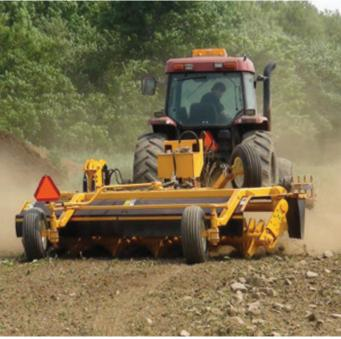
The SWD -15 is designed to adapt to 65-125 HP (48-93 KW) tractors. It digs and moves rocks and roots to form a windrow making them easy to pick up. It is offered in 3 versions.
