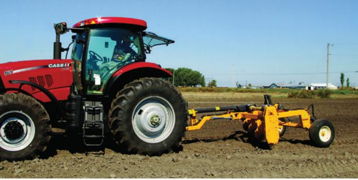
The PWD-10 rock rake is designed to dig and move rocks and roots into a windrow making them easy to collect.
