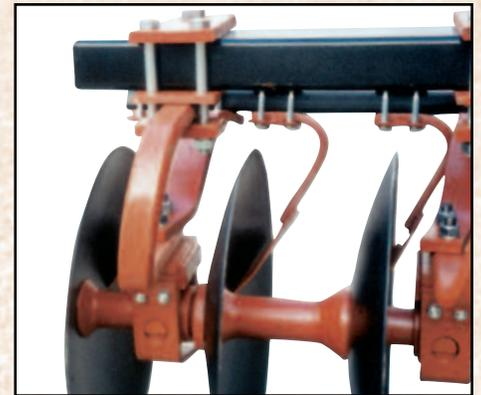
**The Spring Bearing Hanger** provides maximum strength without sacrificing flexibility. It also features a **Wear Plate** which protects the front and bottom of the Bearing Housing.
