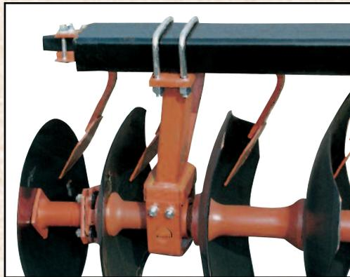
**The Rigid Bearing Hanger** features a **Wear Plate** that bolts onto the front-side of the Bearing Hanger adding extra protection to the front and bottom of the Bearing Housing.
