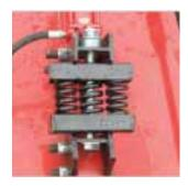
TRIPLE SPRING SHOCK ASSEMBLY (Tailwheel section)
