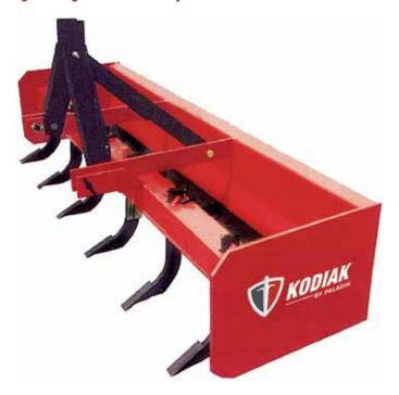
There are 2 weight classes for box blades. Both are ruggedly constructed and are ideal for ripping, grading, leveling, backfilling and general barn lot maintenance.
