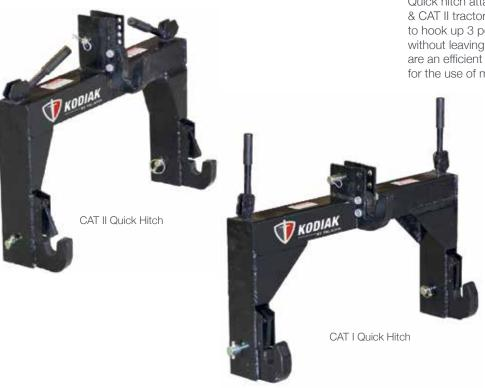
Quick hitch attachments are available for both CAT I & CAT II tractors. These hitches enable the operator to hook up 3 point implements (excluding the PTO), without leaving the tractor seat. These attachments are an efficient time saver when the application calls for the use of multiple implements.
