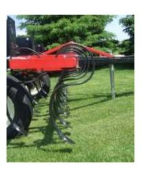
Supported on 7.60 X 15 implement tires. Hydraulic lift is provided by rephasing cylinders with mechanical depth control.
