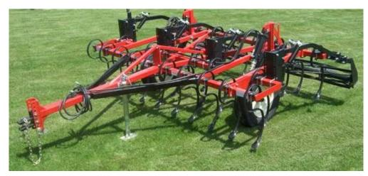
Frame is constructed of heavy gauge 2 ½" X 2 ½" square tubing.
