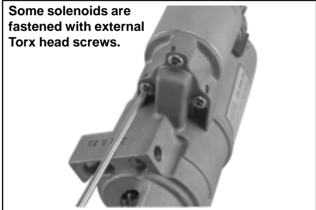
Figure 8-38. Removing Solenoid Screws.
