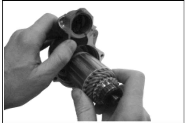
Figure 8-29. Installing Armature.
