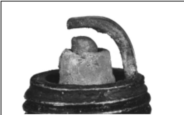
**Worn:** On a worn plug, the center electrode will be rounded and the gap will be eroded .010" or more beyond the correct gap. Replace a worn spark plug immediately.
