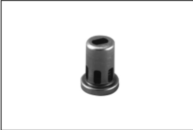
Figure 9-41. Later Style - Oil Pressure Relief Valve.
