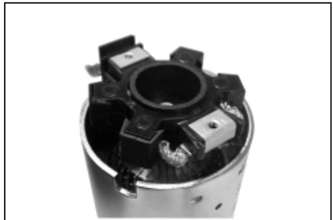
**Figure 8-60. Installing Brush Holder Assembly With Supplied Tube.**
