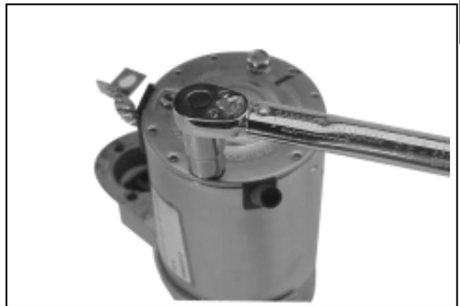
Figure 8-64. Torquing Thru Bolts.
