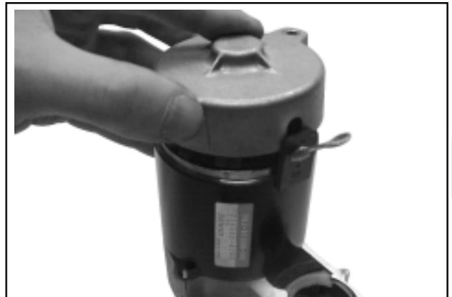
**Figure 8-34. Installing End Cap.**
