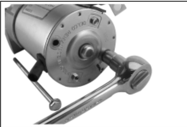
**Figure 8-41. Removing Thru Bolts.**
