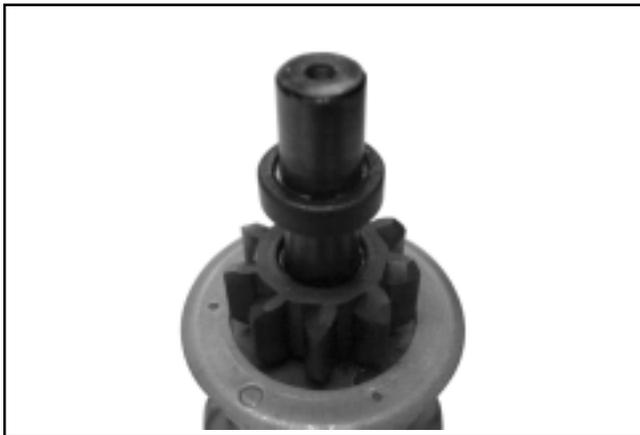
Figure 8-28. Lock Collar around Retaining Ring.
