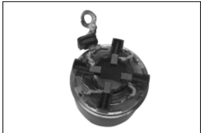
Figure 8-30. Mounting Brush Holder to Frame.
