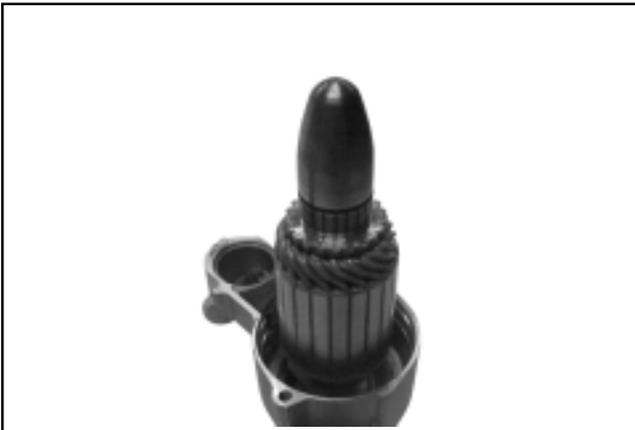
**Figure 8-32. Tool on end of Armature.**
