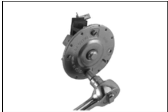
Figure 8-52. Removing Brush Holder.
