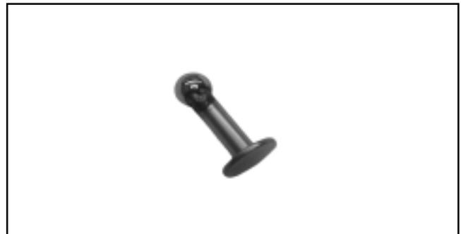
**Figure 11-35. Tappet and Ball Bearing Welded Together.**
