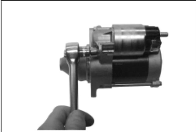
Figure 8-35. Installing Thru Bolts.
