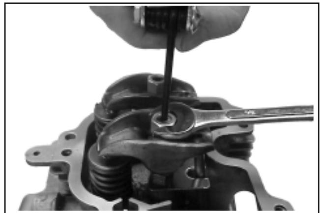
**Figure 11-47. Torquing Set Screw (Adjusting Valve Lash).**
