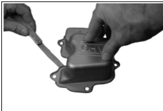
**Figure 10-14. Checking with Feeler Gauge.**
