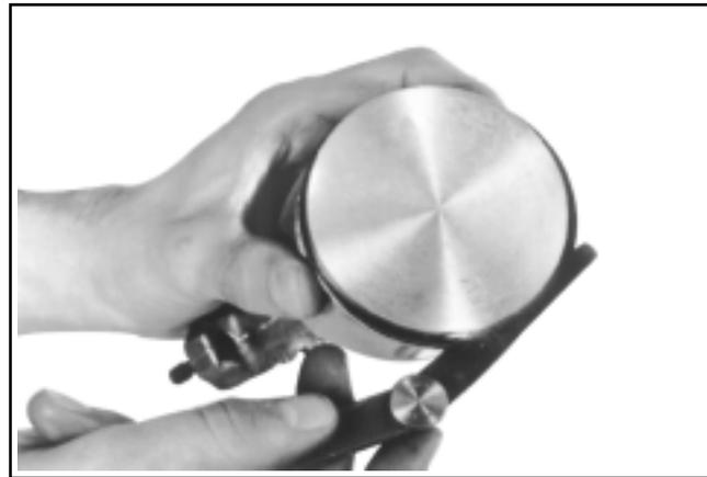
Figure 10-9. Measuring Piston Ring Side Clearance.
