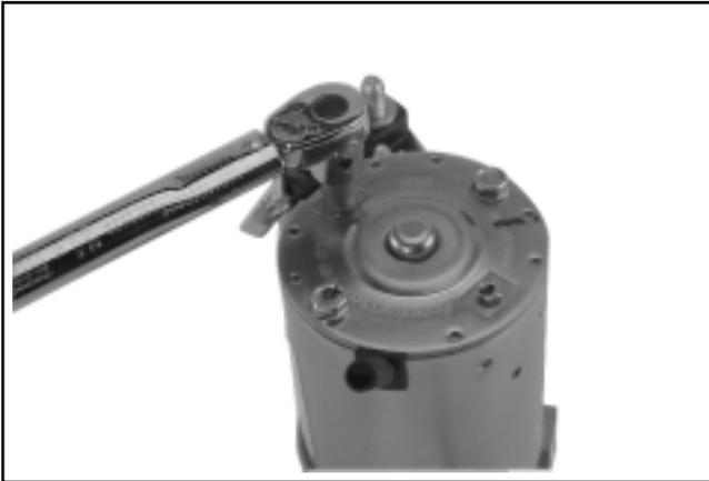
Figure 8-65. Torquing Brush Holder Screws.
