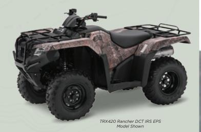
Want the convenience of an automatic transmission, plus independent rear suspension? The TRX420 Rancher DCT IRS EPS gives you Electric Power Steering, Honda's advanced double-wishbone independent rear suspension and Honda's high-tech Dual-Clutch Transmission, which smoothly shifts automatically but has no belts to slip, break or wear out.
