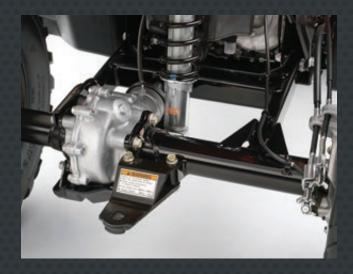
Our workhorse ATVs, plus the TRX90X Youth ATV, employ a durable swingarm rear suspension with a solid axle that's designed to retain consistent ground clearance, enhance roll stability, and ensure predictable handling - all particularly beneficial when riding on sidehills or in other difficult conditions, or when carrying or towing a heavy load.
