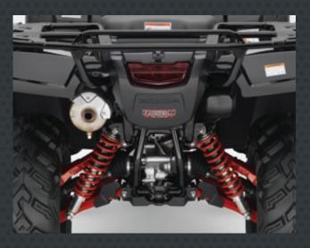
Our trail-focused ATVs come equipped with Honda's advanced dual-arm independent rear suspension (IRS) that provides an extra-smooth ride while maintaining the handling control that all Honda ATVs are famous for.
