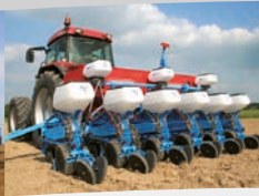
Multi-purpose pneumatic NG Plus 4 planter with discs
