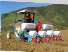
Multi-purpose pneumatic planter with NC shoes
