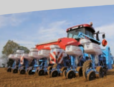
Multi-purpose pneumatic Monoshox® NG Plus M planter with discs
