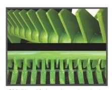
450 BNH steel for heavy duty windrowed picking
