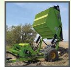
6.5' dump height makes it easier to build larger rock piles
