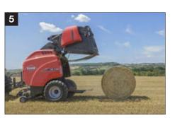
Within 4 seconds the bale is ejected and the tailgate is closed again
