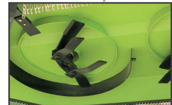
Close up of fixed knife technology with stationary mounted fixed knife and rear mounted baffle
