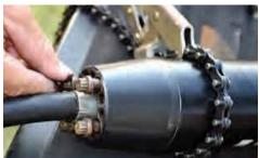
**EFFICIENT TOOL MAINTENANCE.** Tailbolt system provides ease of access for tool maintenance, requiring a maximum of only 35 ft-lb (47.5 Nm) of torque.
