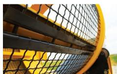
PRODUCT VARIETY. Change product size efficiently with the quick-change screen design. Five large bolts adjust a tensioning hook to allow operators to quickly change screen sizes.
