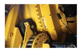
DRUM DRIVE. A hydraulic chain drive system allows the drum to lift off the cog for service. Bolt-on sprockets can be changed quickly and help minimize repair.
