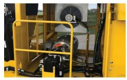
**ELECTRIC MOTORS.** Powered by two industrial-duty, fully enclosed and fan-cooled electric motors. A single 150-hp (112-kW) motor powers the hydraulic pump stack while a .75-hp (.6-kW) motor powers the cooling fan for the hydraulic system.
