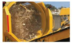
**HIGH PRODUCTION.** The tensioned screens around the drum add rigidity, allowing use of small gauge wire, which helps increase production capacity and enable processing of wetter material.
