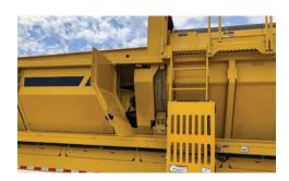
**EASE OF MAINTENANCE.** The TR626EM was built with the operator in mind, designed with various access points to critical areas helping to make maintenance efficient.
