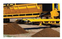
RADIAL STACKING CONVEYOR. The stacking conveyor with a 180-degree arc increases the amount of material being stacked on the ground. Adjustable stacking height aids with dust control and helps avoid material being blown away.
