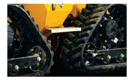
SEE THE DIFFERENCE. When equipped with the innovative quad track system, the RTX550 offers improved flotation, reduced surface damage, increased tractive effort and greater stability. Four-wheel steer and crab steering are functional with the system.
