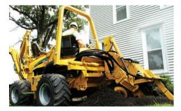
TIRE OPTIONS. The RTX550 is available with standard 31 in (78.7 cm) tires. For even greater flotation, choose the 35 in (88.9 cm) tire option.
