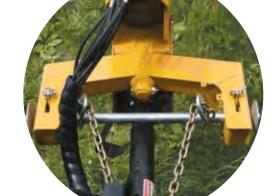
6 A patented 2-point Quick Hitch hookup is designed to allow one person to hook up the mower. It also provides high ground clearance to help avoid obstructions while in the field.
