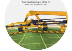
The hydraulic suspension system works in conjunction with the split cutter bar to reduce cutter bar weight on the ground, increase flex and allow the TM1200 to follow ground contouts.
