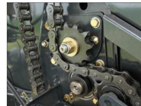
Heavy-duty IWIS chains and hardened sprockets
