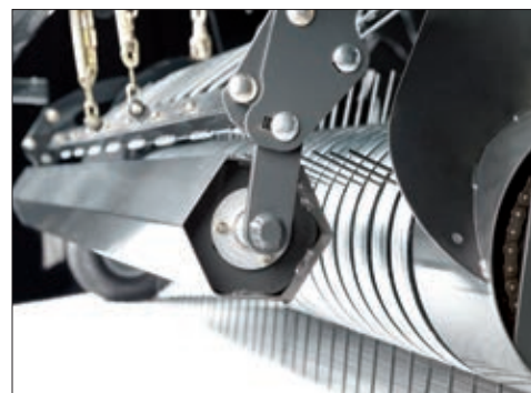
Low-profile, 5-tine bar pickup with standard crop roller
