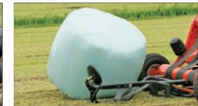
Bale turner gently places the bale on a flat end during unloading (VBP only)
