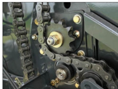
Heavy-duty IWIS chains and hardened sprockets
