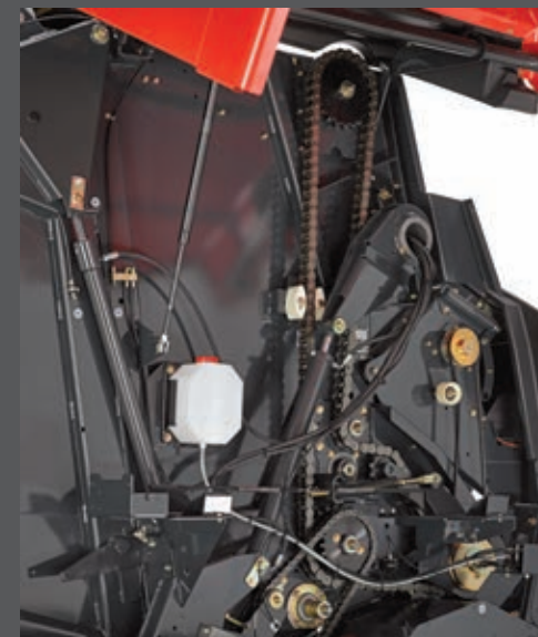
Extremely heavy-duty drive chains
