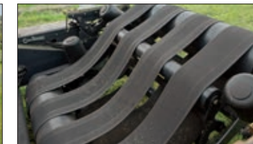
Small bale kit allows you to wrap bales with a diameter of 31.5" and up (VBP only)
