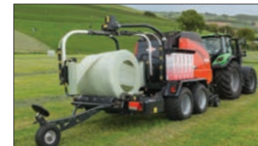
3D wrapping distributes film more more uniformly and efficiently across the entire surface of the bale (VBP only)
