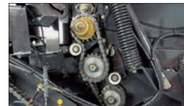
The second drive roller secures bale rotation even in difficult crops (standard on the VB(P) 3165 & 3195)
