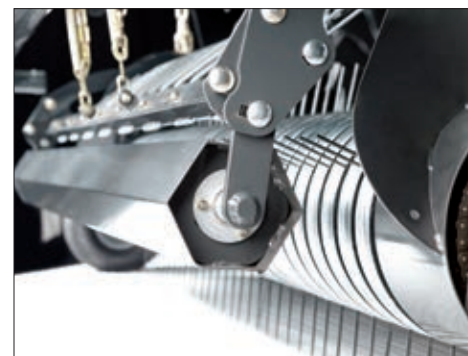
Low-profile, 4-tine bar pickup with standard crop roller
