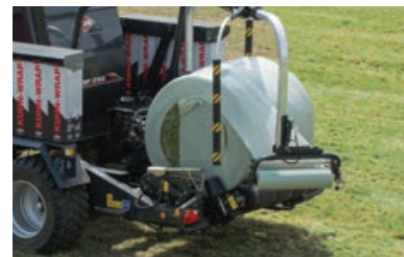
3D wrapping starts by covering the corners of the bale.
