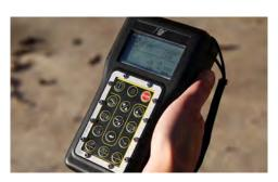
ADVANCE CONTROLS. Operators can control the machine through either the Vermeer DP10 display mounted on the control panel, or through a handheld transceiver remote.
