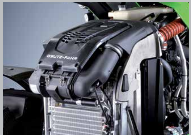
PowerCore technology air filter: 20% higher air flow capacity than comparable standard filters.
