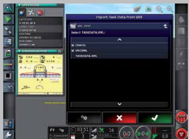
Thanks to the ISOXML standard, tasks can be planned, documented and evaluated with numerous agricultural field records.
