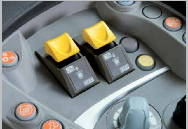
Standard in all cab configurations, the PTO engagement comes with the easy but safe push-button controls.
