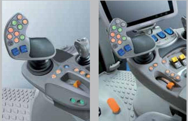
RCshift. The new fully automatic powershift transmission for optimum gear changes.
