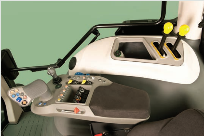
X7 P6-Drive models available in premium configuration feature our premium cab with multi-function controls integrated into the right-hand armrest featuring the latest technology.
