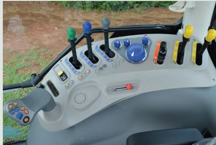
X7 P6-Drive models available in standard configuration feature our efficient cab with multi-function controls integrated into the right-hand console featuring mechanical valve controls.
