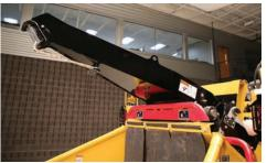
**FEED YOUR WAY.** The patented winch boom design can be raised out of the way when mechanically feeding the machine for optimal visibility and feeding access.
