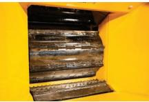
**INTELLIGENT FEED SYSTEM.** Providing over 6,500 lb (2,948 kg) of pull-in power, the AX17 uses SmartCrush and SmartFeed control system that reduces the need for operator interaction when feeding difficult material.
