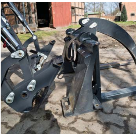
1 Drive up and hook on the front loader
