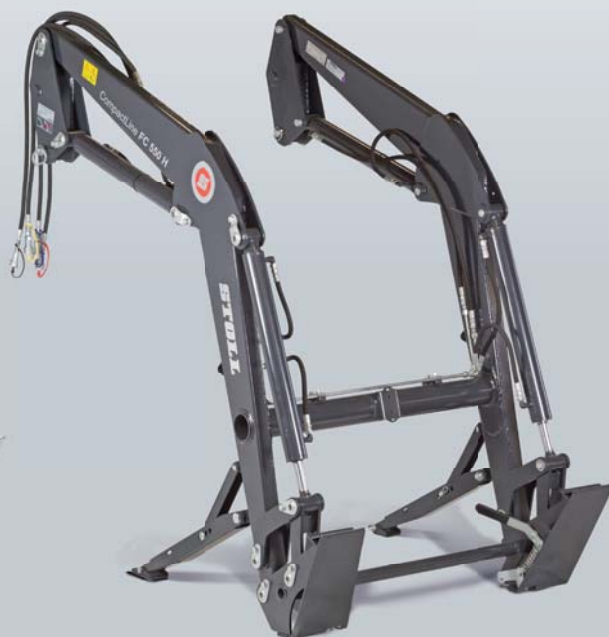
FC-H lift arm without self-levelling
