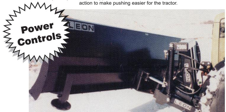
**Power Tilt** is an extra feature that has become a necessity for this heavy duty equipment. Invest initially or add on to the same unit at a later date. The cylinders are positioned to avoid contact with material being dozed.
