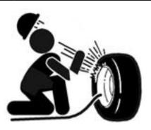
When inflating tires, use a clip-on chuck and extension hose long enough to allow you to stand to one side and NOT in front of or over the tire assembly.
