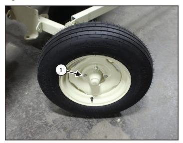
Install the new wheel with the valve stem facing out.
