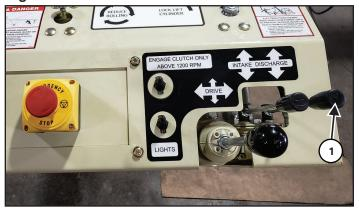
Act on the raise / lower discharge lever (Item 1) at the control console. Use the lever to raise the auger discharge to desired height [Figure 51].
