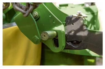
**Contouring across the direction of travel** Elongated holes for the two coupling pins allow the machine to pivot laterally and follow every contour even in the most difficult terrain, providing best protection to the hardware and the sward.
