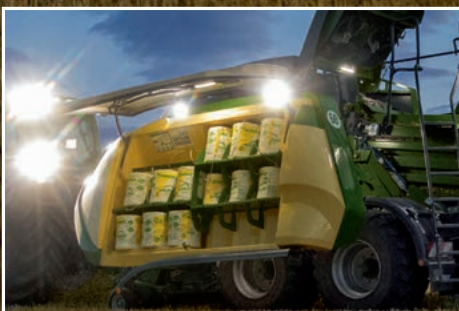
Lights inside the twine boxes
