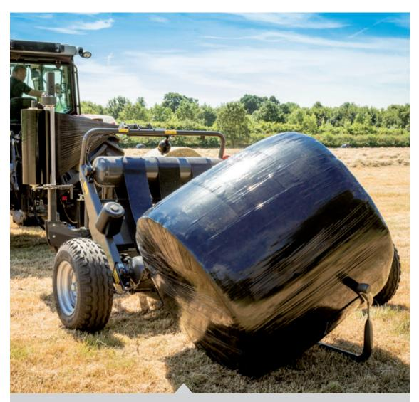
Bale discharge is exceptionally gentle, without the risk of damaging the wrapped bale or the ground, thanks to a low-positioned wrapping table which tilts close to the ground when unloading bales.
