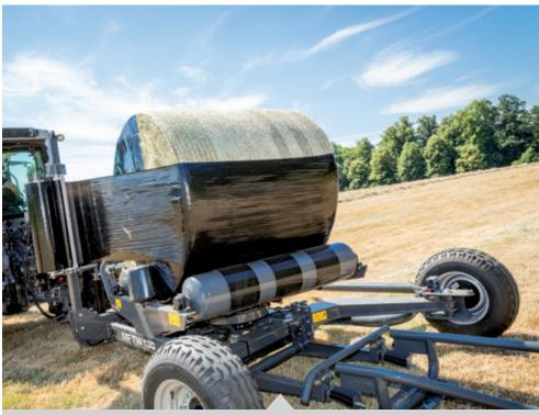
On the MF TW 130 the right-hand side transport wheel can be turned around the centre spindle, extending the overall transport width from only 2.30m to 2.85m, thus increasing the overall wrapper stability.
