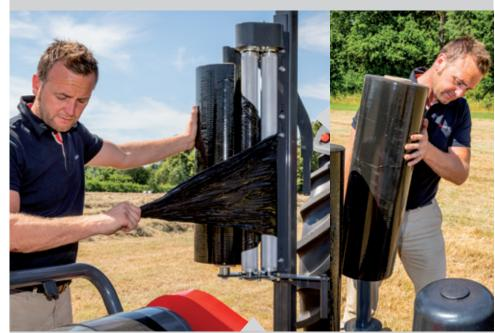
Depending on the crop and conditions, the operator can easily adjust the required number of film layers. The pre-stretching device is designed to work with 500mm or 750mm rolls and can be set at 55% or 70% stretch for tighter wrapping and reduced film consumption. A quick-lock system makes the replacement of empty rolls fast and easy. Storage positions provide the facility to carry up to 3 extra rolls of film.
