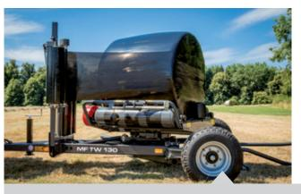
The correct film overlap is ensured by the ratio of bale rotation speed and the speed of the wrapping table. The guides on the wrapping table make sure that the bale remains firmly positioned in the centre of the table.
