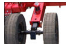
Each axle arm on the center and wings has a spring cushion to absorb the shock loads near the wheel.
