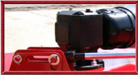
Wing free float is 22° down and 25° up without movement of hydraulic cylinder rod for extended cylinder life.
