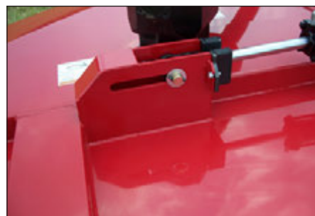
The "free wing float" slot allows the wing to float up and down without moving the hydraulic cylinder rod. This extends the life of the cylinder components.
