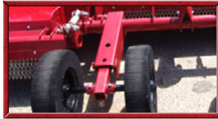
Each axle arm on the center section has a rubber cushion to absorb the shock loads near the wheel.
