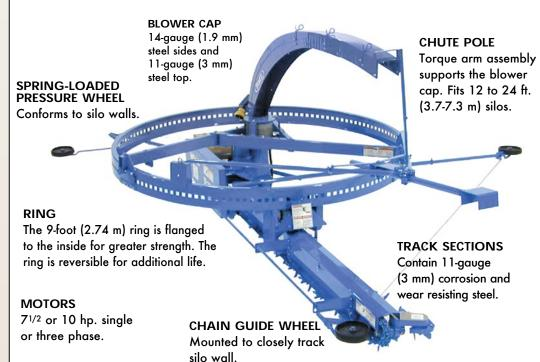
he RD-2200 Silo Unloader combines our aggressive gathering chain in a ring drive. The basic unit adapts to silos 12 to 24 feet (3.7-7.3 m) in diameter by adding a cutter-bar section, gathering chain, guards, and blower cap extensions.
