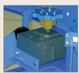
This torque limiter protects the ring and drive gearbox from overload while providing positive drive power (guard removed for viewing).
