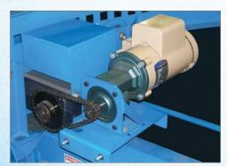
Use independent-motor-drive option if using a center-fill distributor board (guard removed for viewing).
