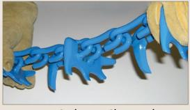
PATZ BLUE Gathering Chain and Sprockets, manufactured using state-of-the-art techniques and a special heat treating process, enable a precise degree of hardening. Includes closed-die forged and hardened cutters and claws for superior strength. The gathering chain's performance results in a high volume delivery for fast feeding. All-welded construction eliminates points of corrosion. Fast (613 ft./min.; 186 m/min) chain speed for high-volume delivery.
