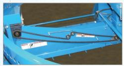
Roller chain drives this RD-2200 around the ring (guard removed for viewing).
