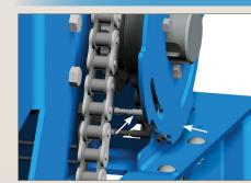
Drive unit design includes sensor disc and proximity sensors to provide the control panel with necessary information to keep track of scraper's position and direction.
