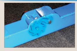
The self-locking ratchet system allows easy tightening of cable.
