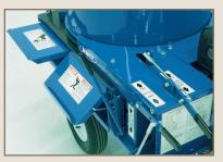
Two adjustable discharge doors direct the flow of materials.
