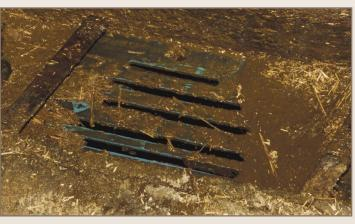
Liquids drop through the screen into the sump. Two screen sizes available: 3/8-inch (9.525 mm) and 5/8-inch (15.875 mm).
