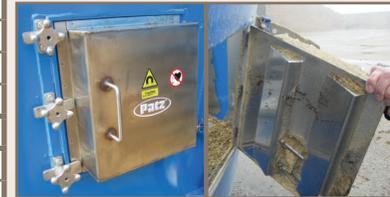
Encased in stainless steel, this magnet is mounted into the Patz Vertical Mixer tub wall on a hinged assembly for effective removal of tramp metal from rations.
