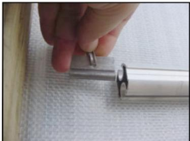
Thread the cable through the clamp then the thimble and the pick-up tab
