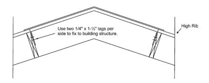
**2.** Using a sheet of glazing you can now space out the remaining trusses along the ridge of the building. Be sure to provide 1/8" of extra coverage of glazing over the truss allowing for expansion. Fix each truss in place using four SN022X5896 Hex Head Lag Scr. SS  $\frac{1}{4}$  X 1-1/2.
