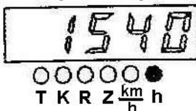
Appearance of the pulses from the speed sensors at the input of the pulse indicator causes the switching-on to the motion speed indication mode. Then the measured calculated speed reading is shown on the digital indicator and the LED located next to the symbol “km/h” lights up.
