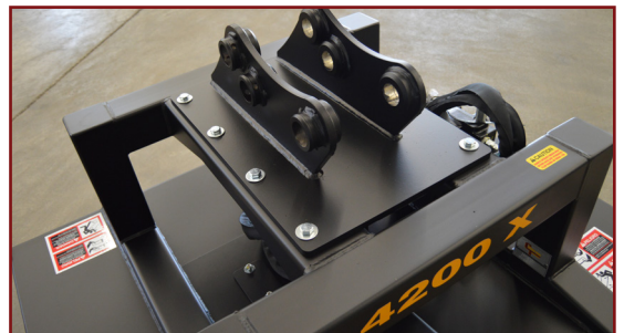
Close-up view of the custom-made excavator hanger
