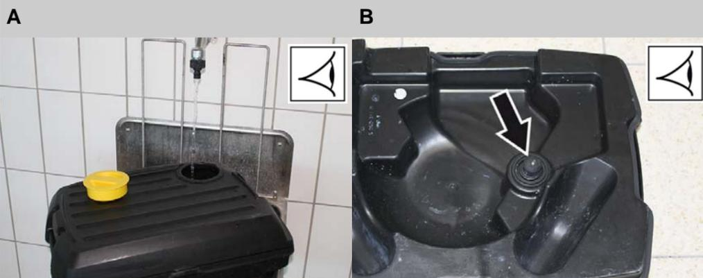
A Fill the fresh water tank with clear water and rinse the appliance to avoid residue buildup.
