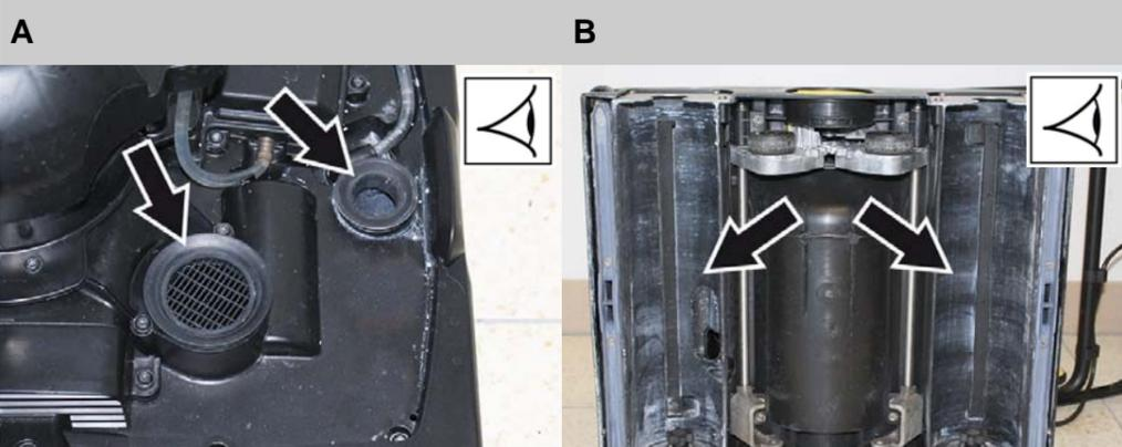
A Check the condition of the seals between the appliance and the wastewater reservoir; replace if required.
