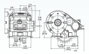
1-Assembly Arrangement with Muncie PKS Series pump mounted to front of PTO. Pump rotation – CW
